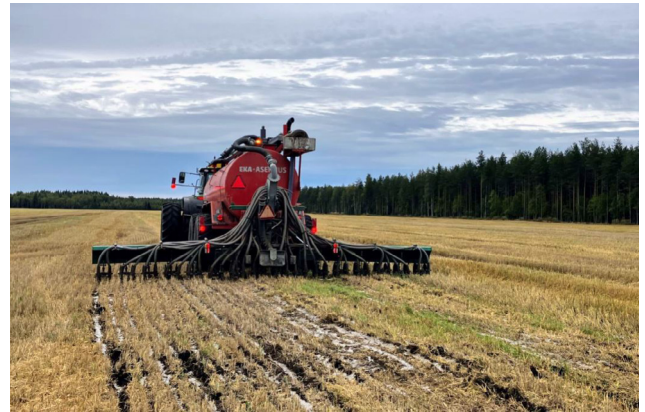
Autumn application of potato starch slurry with an incorporating disc spreader in the "Luomu Ralta" project, carried out in 2020–2022. Photo: Pohjolan Peruna
