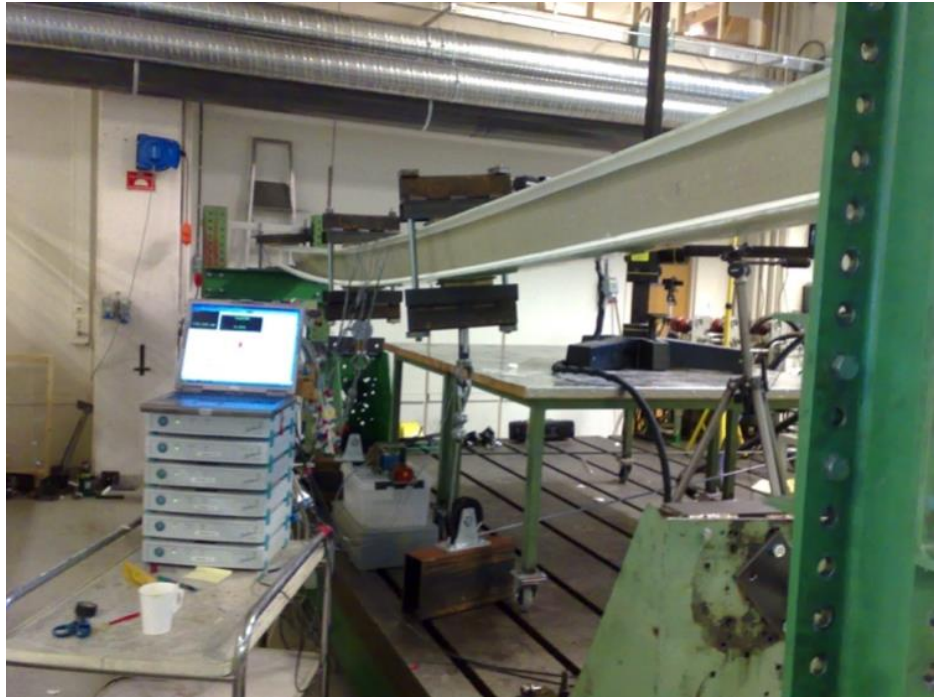
Figure 7 Photo: Bending test of a section on a wing profile. Own photo, from testing
