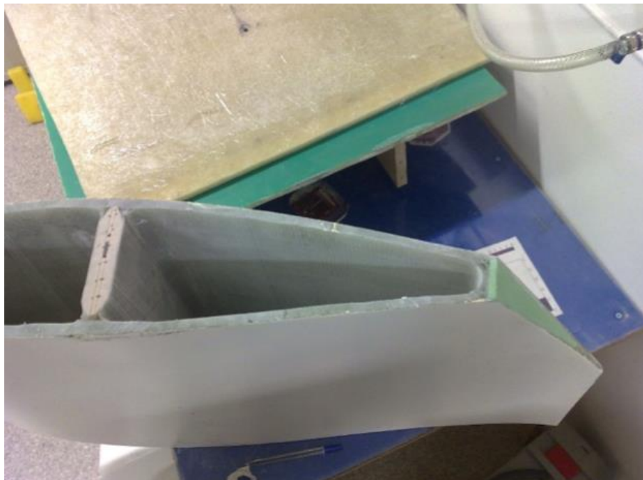
Figure 5 Photo: A small blade profile - to get an impression of proportions. Own photo, from testing
