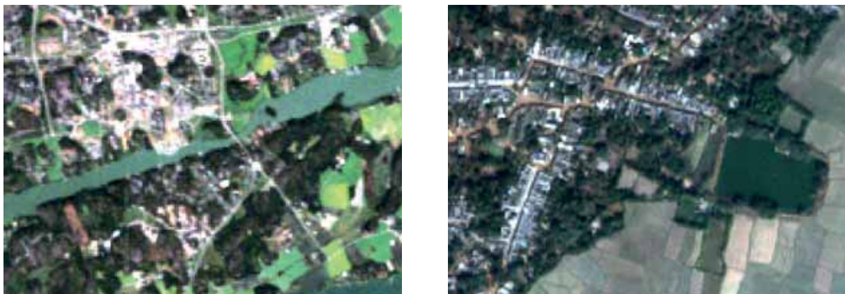
Figure 15. Examples of satellite images: Landsat 5 TM on left (pixel resolution 30 m) and Quickbird on the right (pixel resolution 2,8 m). NASA Landsat Program, 2006, Landsat TM scene L5190018_01820060717, USGS, Sioux Falls, 07/17/2006 (left), DigitalGlobe (2011), QuickBird scene 000000185964_01_P001, Level Standard 2A, DigitalGlobe, Longmont, Colorado, 12/04/2011 (right).
